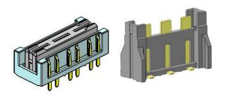
The 10122 series has high voltage rating(600V) / current rating(15A), board to board connector specified for power application. It can cover a wide range of operating temperature. High current rating and a wide range of floating function(self alignment) go well together.
