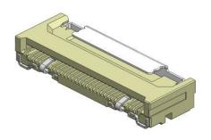
The 11501 Series is a 0.5mm pitch NON-ZIF RA type FFC connector. Compatible with FFC with shield that enables high-speed transmission of digital signals. A shield is attached and EMC measures are also taken.
