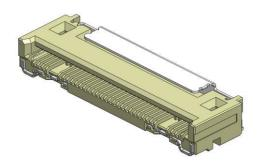
The 11503 series is a 0.5mm pitch NON-ZIF RA type FFC connector. Compatible with FFC with shield that enables high-speed transmission of digital signals. The GND pin is attached and EMC measures are also taken.
