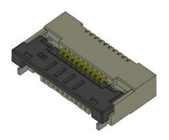
0.50mm pitch, SMT, RA (lower contact) type FPC / FFC connector. Iriso's original lock method I-Lock that thoroughly pursues the prevention of FPC / FFC card disconnection. Front flip structure with good workability. Two-point contact structure with high contact reliability.
