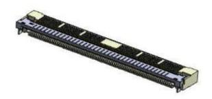
12004S is developed for PCBs between LCD and Touch panel display. Inline connector with 0.4mm pitch is suitable to mount on edge of the board and save space when high pin counts are needed. Features are 2 point contact for high contact reliability and front flip.
