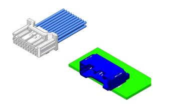
Introducing IRISO's 2.0 mm pitch non-waterproofing connector for in-vehicle device interfaces. The use of 050 terminals (tab size 0.5 mm x 0.3 mm, ultra-compact crimp terminals with box structure) results in a smaller size, lower profile, and higher density. Three types of keying are mounted. Designed for high temperatures; the upper temperature limit is +125C. It is two-row and right angle type with SMT (Surface-mount technology) for automatic mounting.
