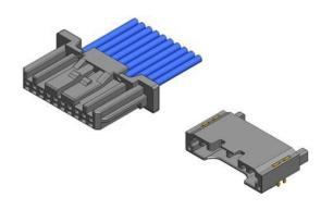
2.0mm pitch non-waterproof Automotive grade interface connector(Header) 050 terminal (Tab size 0.5mmx0.3mm) downsized and low height connector. Operating temperature range us up to +125°C. 1 row/SMT/Right angle version.
