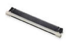
IRISO's 9686 Series is a FFC/FPC connector with a 0.5mm pitch with a slider lock as a secondary locking feature (bottom contact). There are two square cut outs on each side of the FFC which rides over the plastic molded hook from the connector shell (called the I-Lock).
