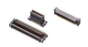
This is a 0.5mm pitch, Board to Board, SMT type connector with a two-point contact mechanism reliability. In case of Iriso's 2-point Contact Connector, the first contact would remove foreign materials (contamination) for better contact reliability. Even if the first contact were on foreign material, the second contact would still be securely touching the contact surface (and vice versa).
